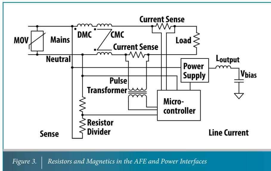
Figure 3. Resistors and Magnetics in the AFE and Power Interfaces
