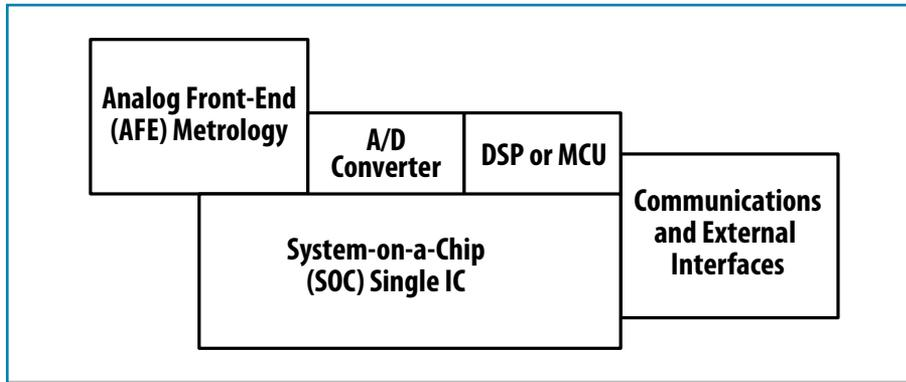
Figure 2B. | Single-Chip Architecture
