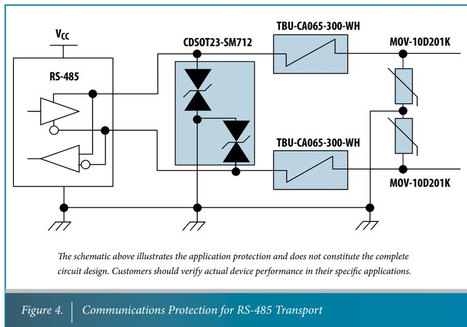
Figure 4. | Communications Protection for RS-485 Transport
