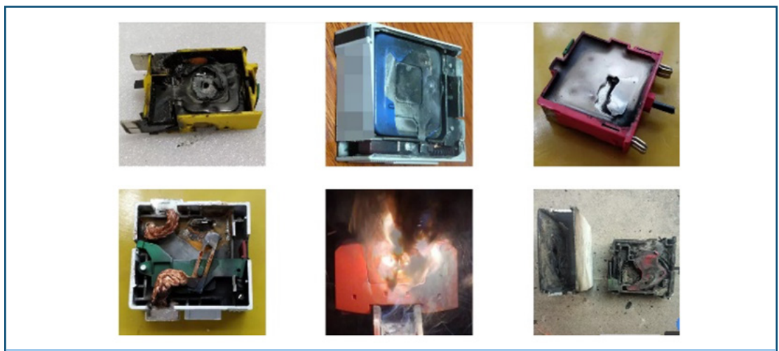
Figure 2. | Examples of overheating and damage to electronics
