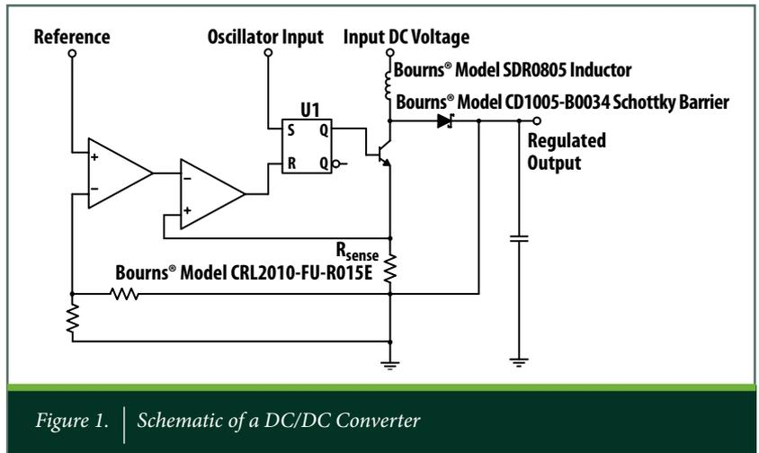
Figure 1. | Schematic of a DC/DC Converter
