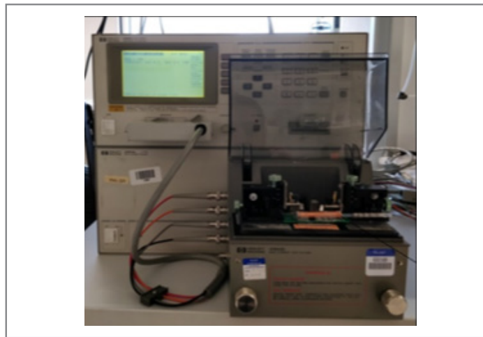
Figure 5: Photograph of the Test Fixture Used to Measure Core Loss
