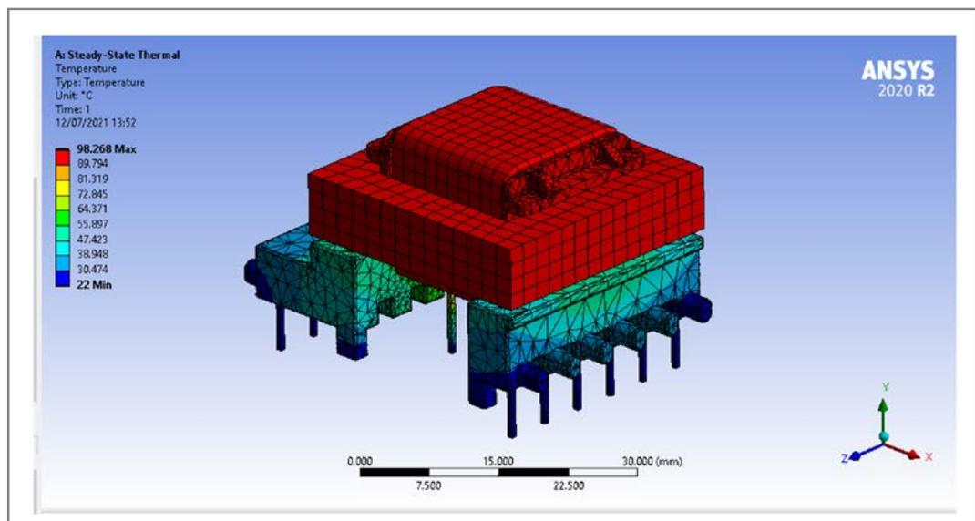
Figure 4 - Ansys thermal analysis for design 1
