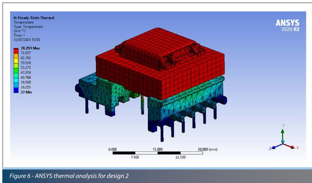
Figure 6 - ANSYS thermal analysis for design 2
