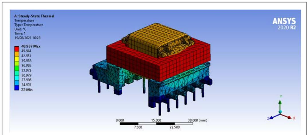
Figure 9 - ANSYS thermal analysis for design 4
