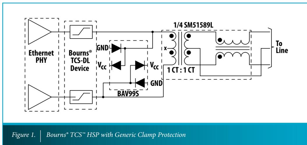
Figure 1. | Bourns® TCS™ HSP with Generic Clamp Protection
