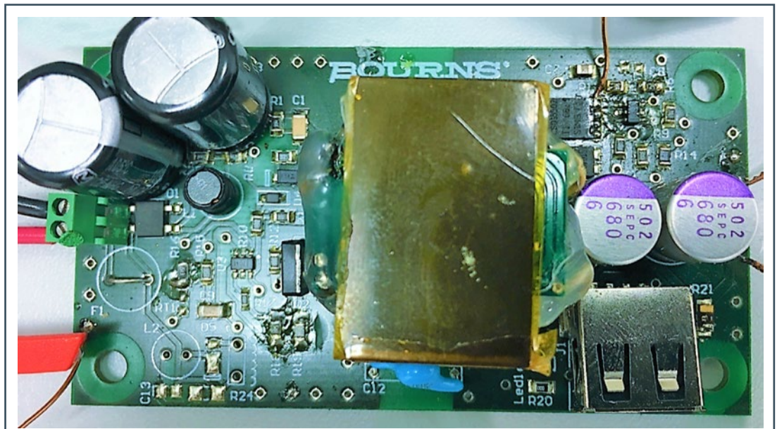
Figure 4. | View of an AC/DC Adaptor with a Planar Transformer and other Bourns® Components
