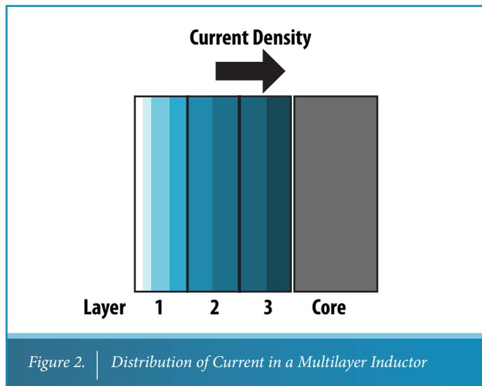
Figure 2. | *Distribution of Current in a Multilayer Inductor*
