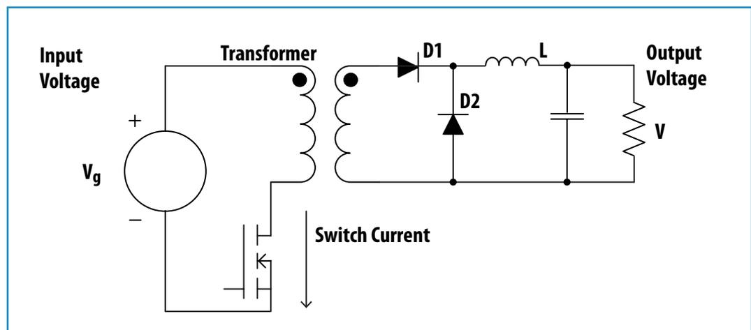
Figure 1. | Basic Block Diagram of Forward Converter Power Stage
