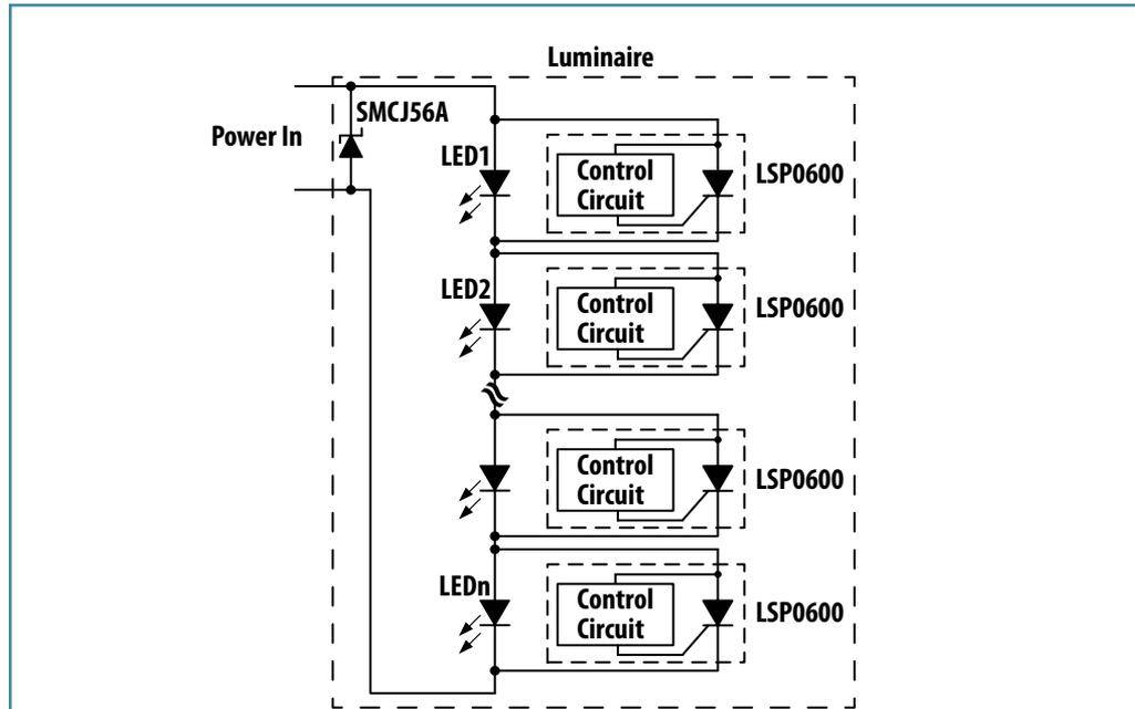
Figure 1. | Optimal Configuration for a Streetlight Luminaire
