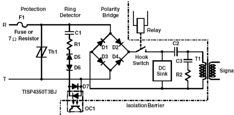
Figure 1. Telephone/FAX Protection
