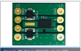
Figure 1a - TBU-RS Series TBU® HSP evaluation PCB.
