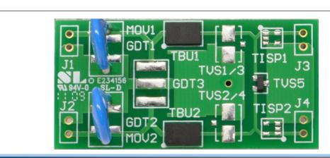
Figure 1b - TBU® HSP evaluation PCB without the integration of TBU® HSP and TVS components into a single device.
