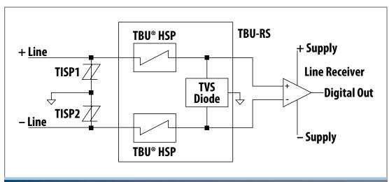
Figure 2 - Bourns® Model TBU-RS Series TBU® HSP with TISP® Overvoltage Protection on an RS-485 Interface.
