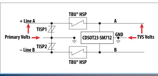
Figure 4 - Bourns® TBU-RS Series TBU® HSP with Bourns® TISP® Overvoltage Protection
