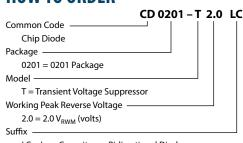
LC = Low Capacitance Bidirectional Diode
