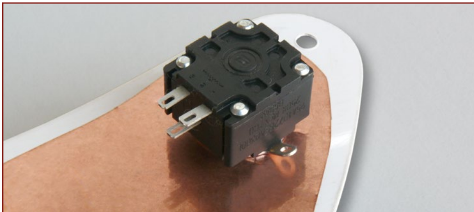
Figure 3: Correct mounting of solder lug lock washer
