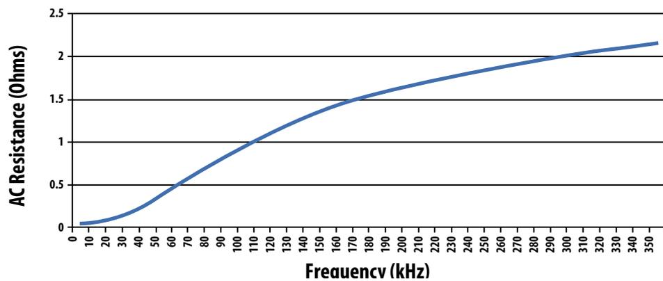
Figure 4. AC Resistance of the Bourns® Model SRR1260-220R0ML Inductor at 40 °C
