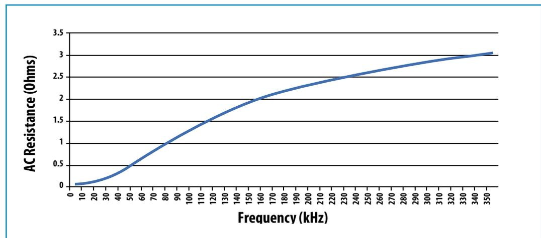
Figure 3. | Dowell Equation Applied to the Bourns® Model SRR1206-220R0ML Inductor
