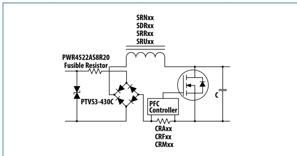
Figure 2. | Streetlight LED Power Supply using a Power TVS Diode
