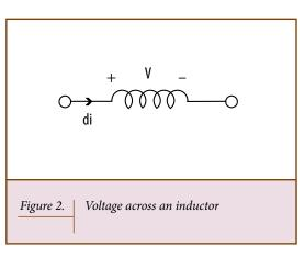
The voltage and current components of the inductor are out of phase such that the voltage leads by 90  $^\circ.$
