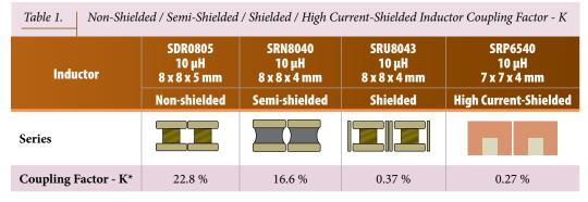
\* Coupling factors of non-shielded / semi-shielded / shielded / high current-shielded inductors in similar sizes are compared at a 100 kHz test frequency with a pair of DUT placed next to each other.
