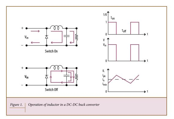
In continuous current mode, the inductor current does not fully discharge to zero during the portions of the cycle in which it is off. A voltage change across the inductor is instantaneous while the current through an inductor varies with time.
