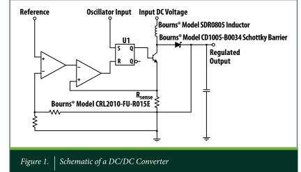
The Schottky barrier diode (Bourns type CD) prevents the capacitor from discharging through the switch to ground. When the inductor current reaches the programmed limit, the switch turns off for a time constant. At the end of the feedback constant, the feedback circuit compares  $V_{out}$  to the regulation voltage and either turns the switch on again (if  $V_{out}$  remains out of regulation) or holds the switch off until  $V_{out}$  falls out of regulation.
