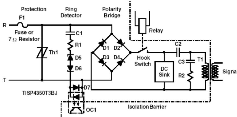
Figure 1. Telephone/FAX Protection
