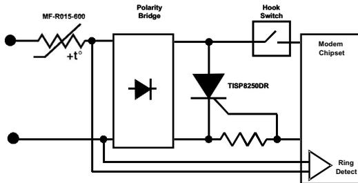
Figure 2. Overcurrent protection
