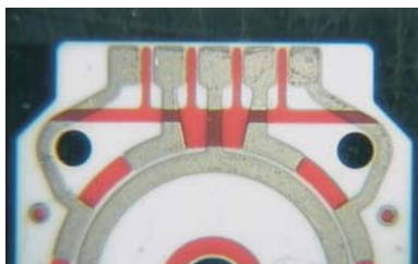
Printed Ceramic Element (Internal View)
