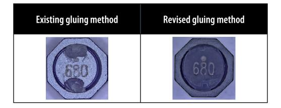
The fit, form and function of the affected part numbers will remain the same. The quality and reliability of the affected inductors should be improved as a result of the changes. The country of origin of the affected part numbers will remain the same. Traceability will be maintained through lot code and date code.
