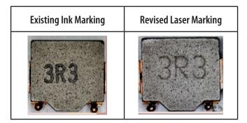
The change in the package cover tape will have no effect on the form, fit or function of the affected models. The change in the component marking method will have no effect on the fit or function of the affected models, but the form will change slightly due to the change from ink marking to laser marking.
