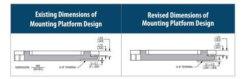
The fit of the inductor will change due to the mounting platform redesign. The form and function remain unchanged. The quality and reliability of the inductor will be improved.
