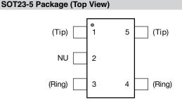
Terminal typical application names shown in parenthesis. NU - Non-usable; no external electrical connection should be made to this terminal.
