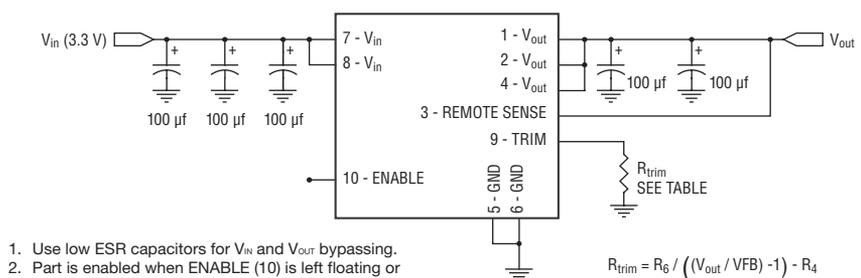
1. Use low ESR capacitors for  $V_{in}$  and  $V_{out}$  bypassing.
