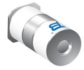
Bourns® Gas Discharge Tubes help prevent damage from transient disturbances by acting as a "crowbar" in creating a short-to-ground circuit during conduction. When an electrical surge exceeds the defined breakdown voltage level of the GDT, the device becomes ionized and rapid conduction takes place. When the surge passes and the system voltage returns to normal levels, the GDT returns to its high-impedance (off) state. RoHS compliant\* versions are available.
