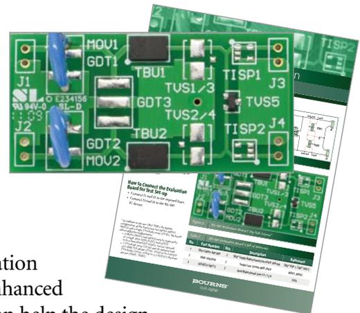
The recommended Bourns® TBU® HSP device solution on both evaluation boards, with a low capacitance GDT on RS-485EVALBOARD1, offers enhanced high-speed performance over competing technologies, which can help the design engineer increase the surge and transient protection level on RS-485 ports and place the entire circuit protection solution into a reduced PCB area.
