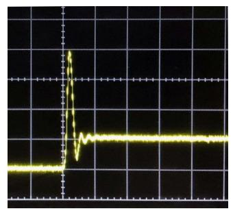
Step response from Fluke 5220A amplifier at 20 A square-wave current (no load), 20 µs/div range
