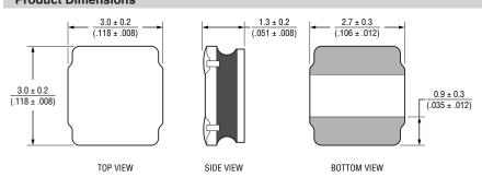
Note: Top and side view dimensions do not include termination. For maximum overall dimensions including termination, add 0.1 mm. DIMENSIONS: (INCHES)
