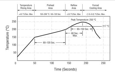
Peak Temperature: 250 ° C max. Max. Peak Temperature -5 °C: 30 sec. max. Time Above 217 °C: 60-150 sec. max.
