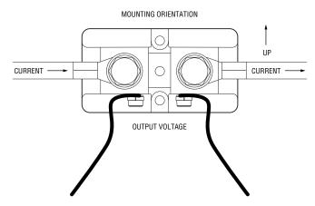
**Operating Current Derating:** For continuous operation, it is recommended that shunts are not operated at more than two thirds (2/3) the rated current under normal conditions per IEEE standards for DC instrument shunts. At ambient temperatures above 40 °C, the current must be further derated to prevent damage.
