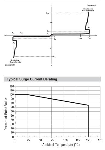
This graph shows the typical device surge current derating versus ambient temperature when subjected to the 8/20  $\mu$ s current waveform per the IEC 61000-4-5 specification. This device is not intended for continuous operation at temperatures above 125 °C.
