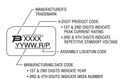
**How to Order** PTVS 1 - xxx C - T H L Series PTVS = Power TVS High Current Diode Peak Current Rating 1 = 1 kARepetitive Standoff Voltage 066 = 66 V 190 = 190 V 380 = 380 V Suffix -C = Bidirectional Device Package T = Through-Hole Temperature H = High Temperature Series Blank = 5 pcs./tray
