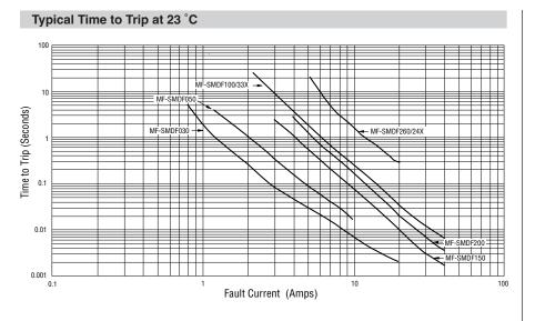
The Time to Trip curves represent typical performance of a device in a simulated application environment. Actual performance in specific customer applications may differ from these values due to the influence of other variables.
