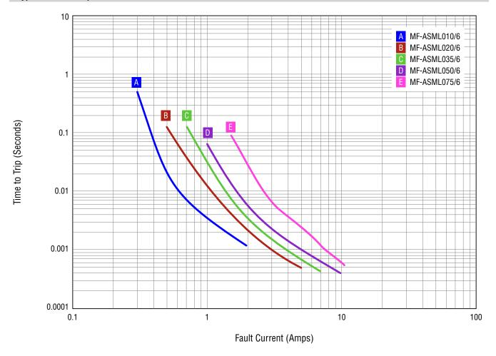
The Time to Trip curves represent typical performance of a device in a simulated application environment.
