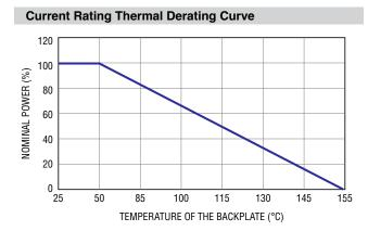
The PWU220 resistors must be attached to a suitable heat sink. The maximum internal resistor temperature is  $+155\,^{\circ}$ C.
