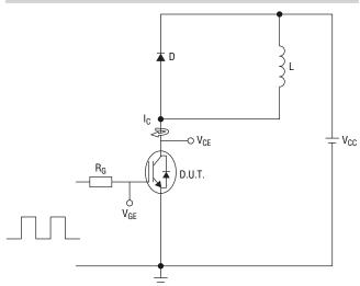
L = 2.8 mH,  $V_{CE}$  = 400 V,  $V_{GE}$  = 15 V,  $I_{C}$  = 20 A,  $R_{G}$  = 10  $\Omega$
