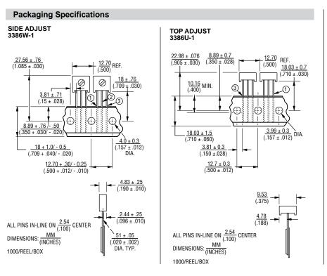
3386 P-1-103 T Model Style Standard or Modified Product Indicator -1 = Standard Product -EY5 = Extended Shaft Resistance Code Optional Suffix Letter  $T = Knob^*$ Packaging Designator
