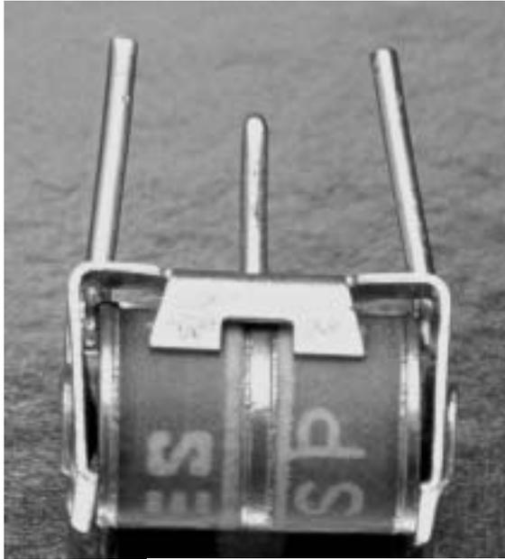
With the failsafe activated, the tin/lead plated electrical grade contacts are held closed by spring tension. This creates a dead short from each input to ground of less than ten milliohms. There is neither an insulation burn through media that can degrade contact resistance, nor is there a compressed solder pellet which can create thermal cycling problems.
