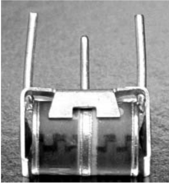
The failsafe mechanism consists of spring loaded tin/lead plated electrical grade contacts. The outer clip is electrically connected to the gas tube center lead. The inner conductor is the gas tube end electrode. The spacing between the contacts is set to be greater than 0.010 inch (typically 0.015-0.020 inch). There is no insulating media between the contacts, which could absorb moisture or become contaminated.
