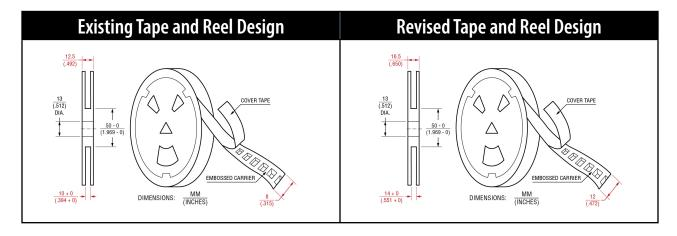
The form, fit, and function of the inductors will not change as a result of the changes to the carrier tape and reel. The quality and reliability of the inductors should be improved with the above changes. Traceability will be maintained through lot code and date code.
