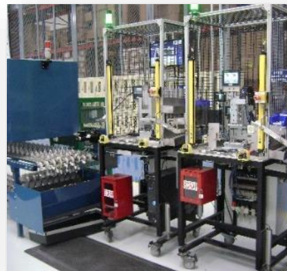
Bold insert station & screw installation
